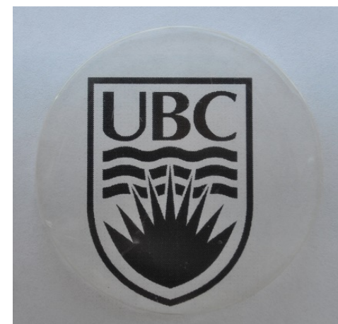
Figure 2. Transparent chitosan bioplastic on a paper UBC logo
